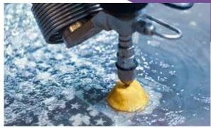
Waterjet Cutting machine capabilities up to 100 mm for steel, Stainless, Aluminium and Polycarbonate material.
