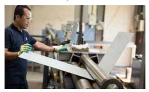
Pressbreaks can fold up to 3m long, max 15 mm thick for steel. CNC rolling from radius 60-1500 mm, max thickness 4 mm for steel.
