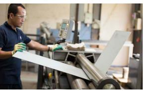
Pressbreaks can fold up to 3m long, max 15 mm thick for steel. CNC rolling from radius 60-1500 mm, max thickness 4 mm for steel.
