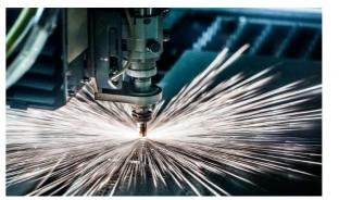
Fiber Laser cutting capabilities up to 20mm thick for steel, 10mm for SUS/ AL. Tube laser can cut steel tubes up to 150x150 mm.
