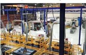
High pressure cabinet leak test stations with overhead gantries.
