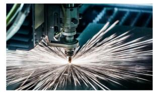
Fiber Laser cutting capabilities up to 20mm thick for steel, 10mm for SUS/AL, Tube laser can cut steel tubes up to 150x150 mm.
