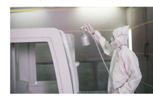
Automotive quality wet paint booth can handle parts up to 2m tall. External suppliers for a wide variety of industrial coatings.
