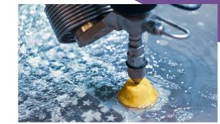
Waterjet Cutting machine capabilities up to 100 mm for steel, Stainless, Aluminium and Polycarbonate material.
